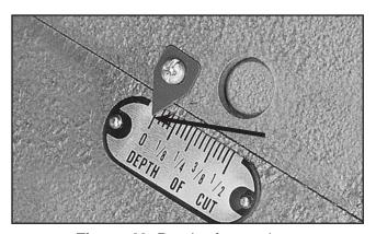
**Figure 46.** Depth-of-cut pointer adjusted to "0" position.
